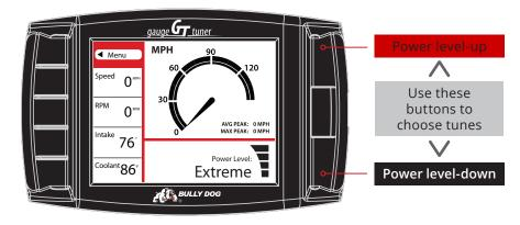
That is when you will have the option to use the switch on-the-fly feature. Initially, the tuner will be in safety warm-up mode and once the truck hits the correct temperature, you'll see the options for the SOTF, in the bottom right corner.
